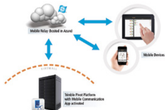
Illustrating the workflow between the Trimble Mobile Communication App, relay server and the Trimble mobile apps.
