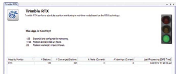
Pivot RTX App Status View on the Trimble Pivot platform
